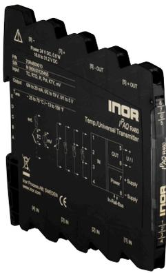
IPAQ R460 is a programmable 4-wire (separately powered) transmitter. It converts Pt, Ni, KTY and TC sensor signals as well as potentiometer, resistor and mV signals to isolated standard signals.
