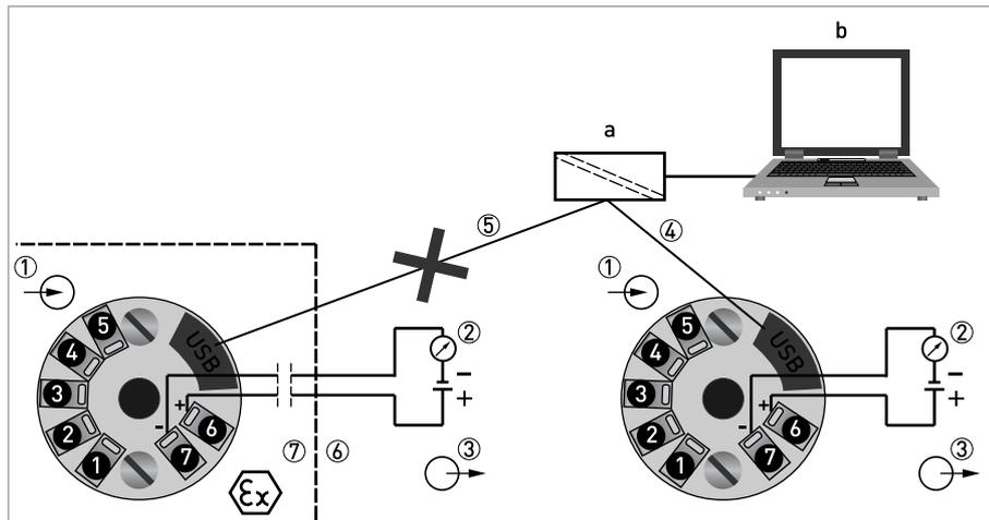
Figure 5-1: Connection during configuration of in-head transmitter
