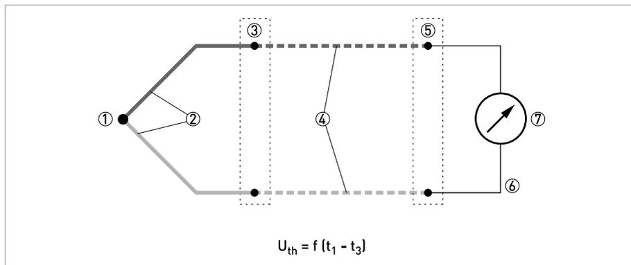
**Figure 7-2: Thermocouple measuring circuit, schematic**
