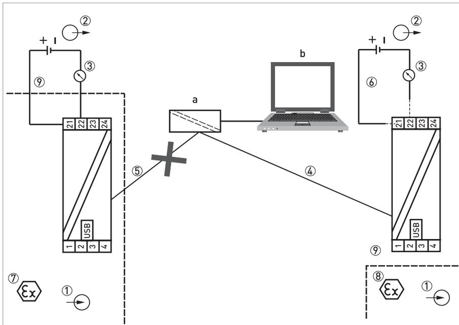
Figure 5-2: Connection during configuration of rail-mount transmitter
